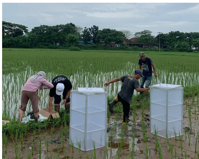
Methane concentration measurement in a rice paddy implementing AWD (Indonesia)
