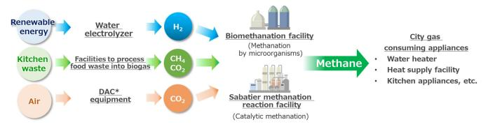
$\mbox{\%DAC(Direct Air Capture):Direct CO2 capture technology from the atmosphere}$
