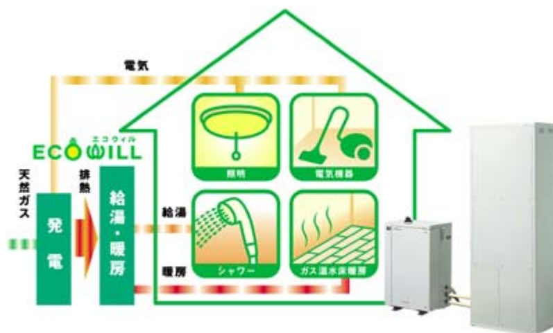
residential gas cogeneration system "ECOWILL"
