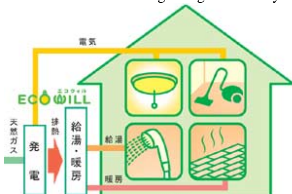
Mechanism of “ECOWILL” which generates electric power by using natural gas and uses exhaust heat from such electric power generation for hot water supply and heating
