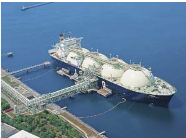
LNG being unloaded from a tanker
