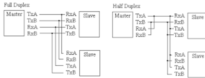
Figure 4. Schema of half duplex and full duplex.
