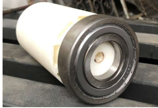
Figure 4 (a) The top view of the prototype, (b) three bins that function to collect three different categories of materials, (c) the splitter that can be adjusted for fine tuning during the process of separation, and (b) the 3D-printed drum which contains eight pieces of permanent magnets
