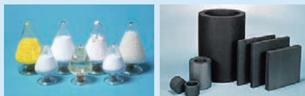
Fluorene derivatives (left), used for lenses and other applications in the optoelectronic field, and sectional insulation (right), an activated carbon fiber
