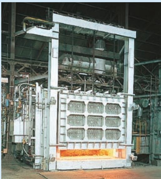
Regenerative burner system that realizes high-efficiency, energy-saving fuel combustion for industrial furnaces
