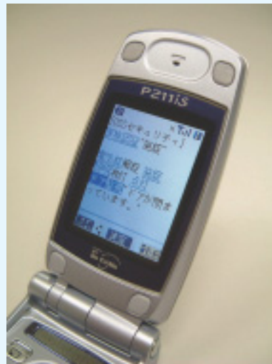
I-rusu enables use of a mobile phone to control or check on lighting, underfloor heating, hot water supply and other home utilities. (Osaka Gas Security Service Co., Ltd.)
