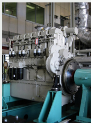
Long-stroke Miller-cycle gas engine boasting a generation efficiency of 42%
