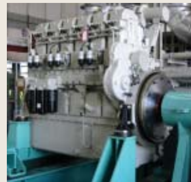
Long-stroke Miller-cycle gas engine boasting a generation efficiency of 42%
