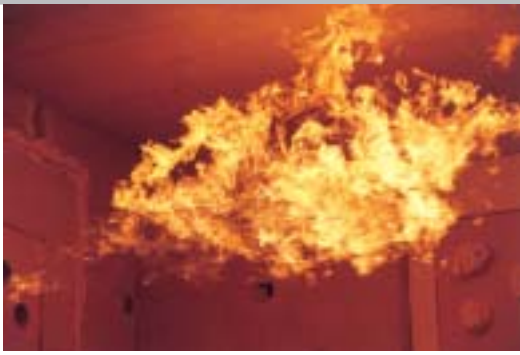
Regeneburners enable reductions in energy consumption of 35-50% using the accumulated heat burning method.
