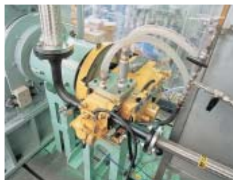
This gas engine incorporates compressed auto-ignition technology.
