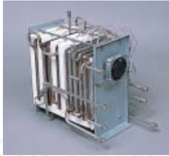
This gas reforming equipment extracts hydrogen from natural gas.
