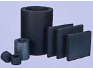
Heat-resistant materials using carbon fibers manufactured by Osaka Gas Chemicals.
